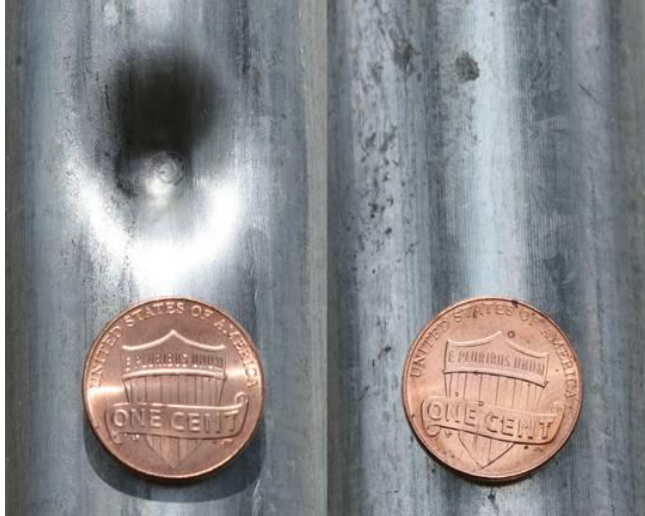
Handgun (.22) bullet damage to a metal pipe Left picture is the front of the pipe. Right picture in the back of the pipe.
