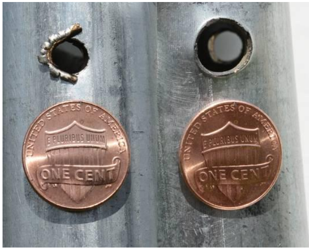
Assault rifle (.223) bullet damage to a metal pipe. Left picture is the front of the pipe. Right picture in the back of the pipe. Photo credits above: Aaron Spuler
